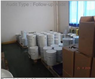
External photo(s) of the production unit(s) 7-7 Safety label posted but without secondary container.JPG
